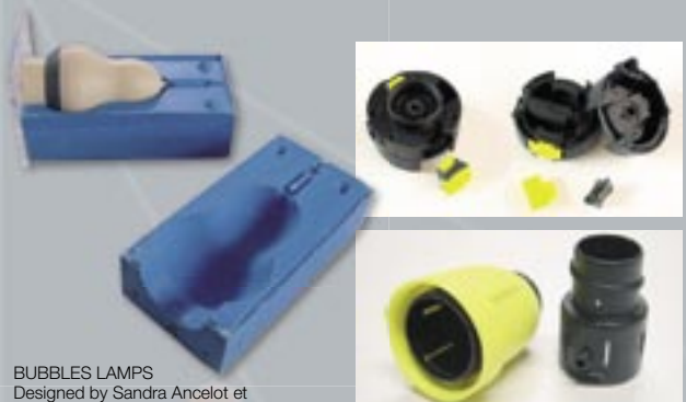
REGULATOR OF OXYGEN TANK Functionnal parts. Example of vacuum casting, high precision parts, including different types of products ABS and rubber like. AEF Design for Fenzy
