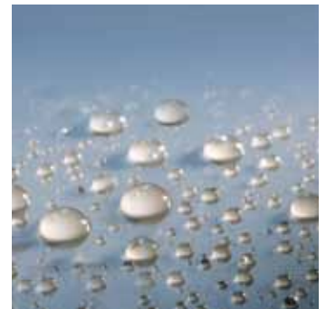
After 1 day: complete recovery of hydrophobic surface
