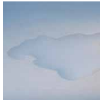
After plasma treatment: hydrophilic surface
