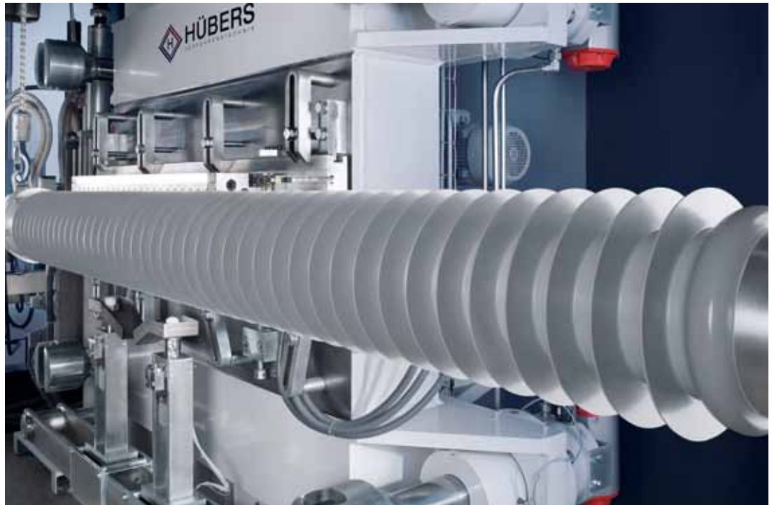
220 kV hollow insulator made by Hübers – with courtesy of Hübers, Germany
