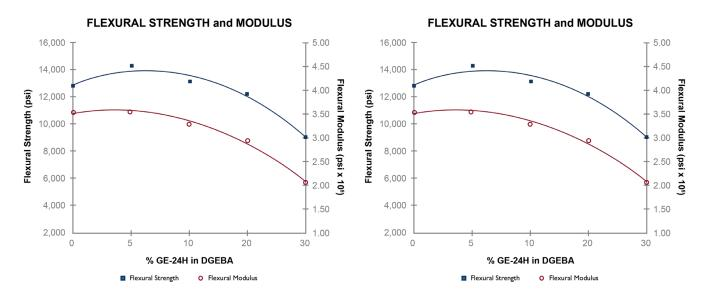
The effect of ERISYS® GE-35H resin on the cured properties of liquid epoxy resin (EEW 188) cured with Polyamidoamide for a flexibilized formulation.
