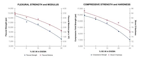
The effect of ERISYS<sup>®</sup> GE-36 diluent on the cured properties of liquid epoxy resin (EEW 188) cured with Polyamidoamide for a flexibilized formulation.
