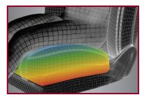
This next generation seating foam technology by Huntsman is completed in one pour, with one formulation. Huntsman's RUBIFLEX® Gradient Hardness™ polyurethane system provides optimal comfort for the driver and minimal steps in the manufacturing line, thus saving automakers time and money to deliver a level of comfort previously only experienced with premium seats.
