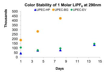
In 1M LiPF<sub>6</sub> in **ULTRAPURE® EC**:EMC (1:2 v/v), **ULTRAPURE® EC-EV** and **ULTRAPURE® EC-HP** demonstrated the best color stability and performance.
