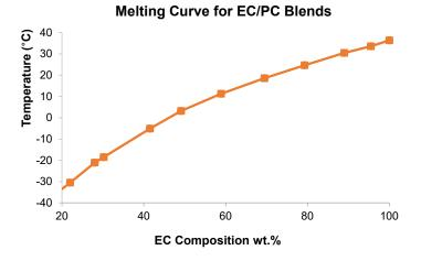
The freezing point of **ULTRAPURE® EC** can be depressed by blending with **ULTRAPURE® PC**, which improves product handling. The melting curve above illustrates the melting point changes in **ULTRAPURE® EC/PC** based on the composition of the blend.
