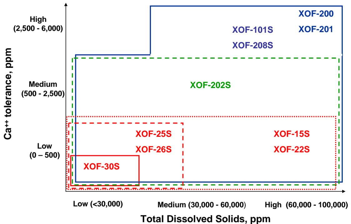
For alkylaryl sulfonates, the hardness tolerance remains relatively low regardless of molecular weight. As shown in Figure 3, these surfactants must be blended with co-solvents and co-surfactants in order to expand their useful TDS and hardness range. In applications that involve reservoir temperatures less than 80°C, the sulfosuccinate co-surfactants XOF-200 and XOF-201 work very well.
