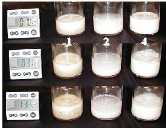
Although blends 3 and 4 were made with the same Suprasec 2408, the test shows that the stability of the blend depends on the mix ratio isocyanate/water. Due to the small amount of water in blend 3 (mixture 95/5), the dilution is limited and the carbon dioxide produced makes the system foam rapidly.
