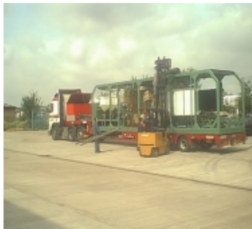
Figure 7 : Slabstock module during dispatch at Cannon Viking, Manchester, UK. This module houses the fall plates and mixhead, control and electrical panels, additive tanks and pipework local to the mixhead. Bottom and side paper handling equipment is included.
