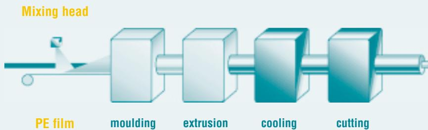
pipe is necessary. Because of the good distribution of the foam, the filling density can be reduced considerably. Also the thickness of the HDPE casing pipe can be reduced significantly, in particular for larger diameters, as it does not have to withstand a high pressure resulting from the foam expansion.
