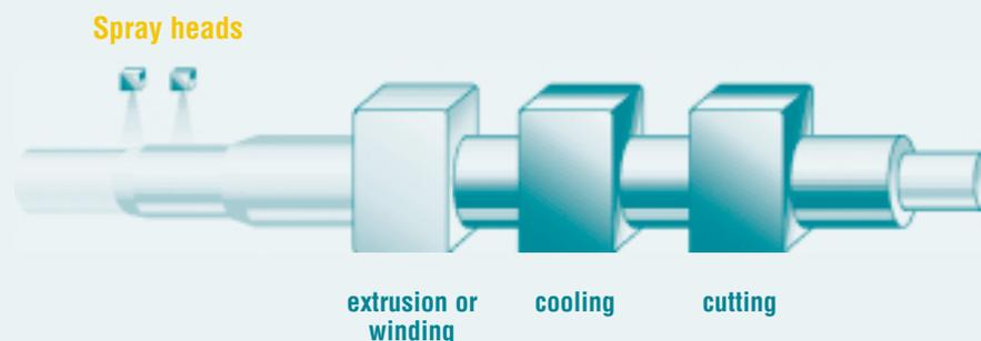
The foam surface is not completely smooth. In practice, the spray technique is only suited for big diameter pipes. Losses caused by overspray restrict this technique to bigger diameter pipes where the waste generation is limited.
