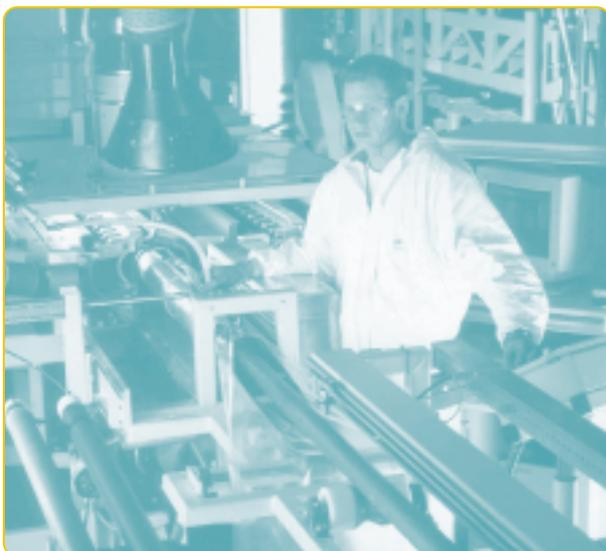
The continuous moulding technique can be used for flexible and rigid pre-insulated pipes. Different service pipes, i.e. made with cross-linked polyethylene, polybutylene, aluminium, copper or steel can be employed. Because of the importance of this technique, we have invested in a small scale continuous moulding machine in order to enable us to develop and optimise foam systems for this manufacturing technique.
