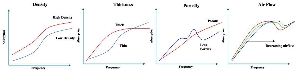
Summarising the effects highlighted in the graphs increasing density / thickness / porosity and airflow<sup>vi</sup> will result in increased levels of absorption performance and with that the potential to improve the acoustic comfort of any space that these materials are used within.
