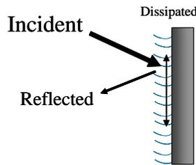
The reflection coefficient of a surface is defined as the ratio of reflected sound to incident sound in the following manner.
