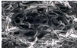
**ACOUSTIFLEX<sup>®</sup> S @ Density 15 kg/m<sup>3</sup>**
