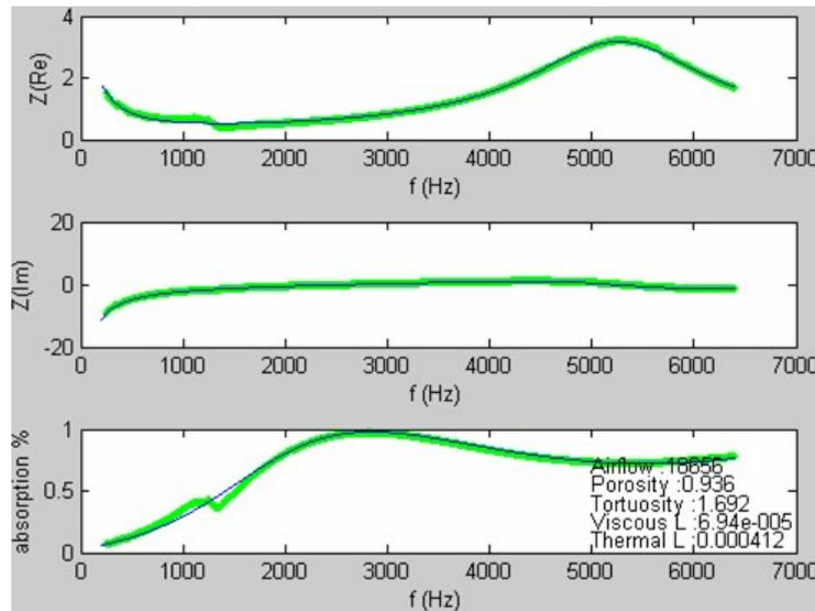
Using these values it is then possible to determine the impact of various factors on the performance of the foam systems. In addition to the impact of physical characteristics it is also possible to model the impact of various types of measurement conditions on the performance of the system. The example shown below highlights the difference between oblique & random incidence (see figure 6).
