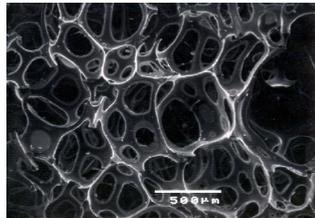
**Conventional Flexible Foam @ Density 40 kg/m<sup>3</sup>**
